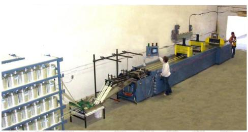
The current sign infrastructure uses posts that are 2 inches by 2 inches and the pultrusion system produces these in 2 or more lines through the pultrusion system at the rate of 4 feet per minute minimum. Posts can be produced to any length and standard saws used
